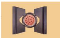
If the force is applied on opposite sides (only two pressure points), the shell will tend to collapse, and this will in turn produce false torque readings because of increased friction between the components where the threads have been forces together.
