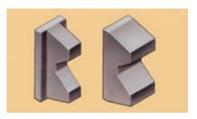
Jaws are available in two gripping widths: .400" and 1.000". the narrow jaws allow access to accessories which are smaller in diameter than adjacent components, whereas the wider allow for a large grip area when higher torque values are required.
