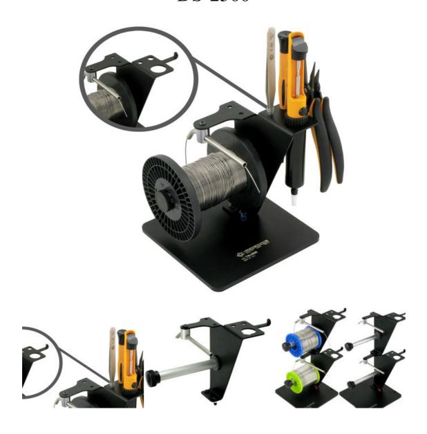
Keeps the working area tidy and reduces solder waste through a guiding tube. In the back of the dispenser it is possible to insert different hand tools to be used by the operator while soldering (such as soldering pump, tweezers, pliers or screwdrivers). It can be positioned in such a way that the hands of the operator are free to use soldering iron and components.
