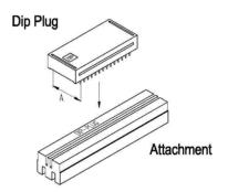
: For Crimping DIP-PLUG Distance A - 0.1" 0.3" & 0.6" (Within 40 Pins)
