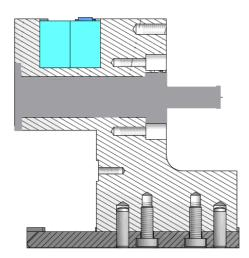
The integrated cylinder in the basic body allows feed settings for terminals up to increments of 50 mm without excess of the dimensions of customary pneumatics applicators.
