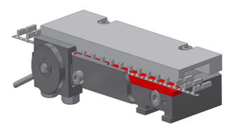
The adjustable table is pre-position in the suitable position for the terminal and is screwed with a block on the baseplate. Afterwards the table can be postadjusted by the additional possibility of adjusting of  $\pm$  4 mm and the table is put in the exact position to the anvil. Due to its unique system the table can be adjusted in a quick, precise and easy manner.
