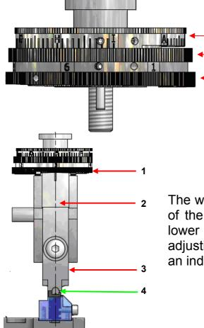
The wedge (2) and thereby the pressure piece (3) of the cutting time (4) is adjusted by turning the lower adjusting disc (1). The setting of the adjusting disc in increments of 0.02 mm permits an individual optimization.
