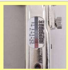
The **612118** can be adjusted and set at crimp depths ranging from .015-.043 inches, with increment settings of .0005
