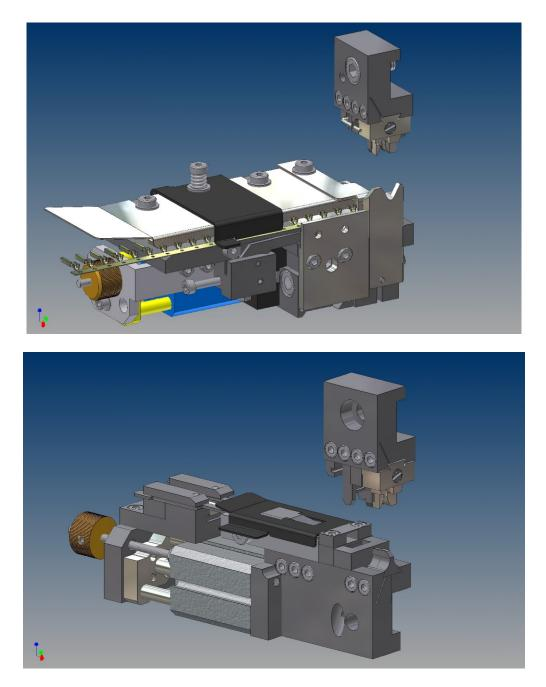
This crimp tools can used for Kirsten PP-3 and AWM 3PP. The feed works with pneumatic cylinder. Maybe you need the optional pneumatic kid to connect the tool with the machine.
