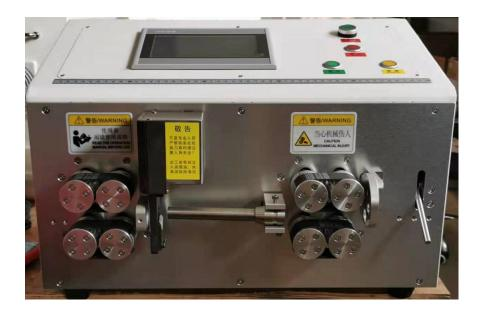
This machine adopts 8-wheel drive with powerful and precise dual-side pressure rollers. Its belt feeding system ensures no damage to the surface of the wire. It is widely used in the processing of military, medical, communication, power cables, sheathed wires, and both soft and hard wires.
